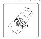
Remove batteries from remote control
