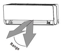
**NOTE:** Do not move louver by hand. This will cause the louver to become out of sync. If this occurs, turn off the unit and unplug it for a few seconds, then restart the unit. This will reset the louver.
